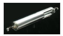
These helium-neon laser tubes have two Brewster windows with external cavity mirrors. This configuration is ideal for applications, such as particle counting, that requite access to the high intra-cavity power. These lasers provide all the benefits of a high power laser without the high cost.
